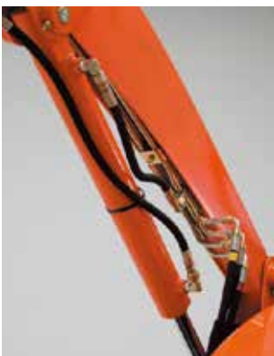
Protected Cylinder Tubes
