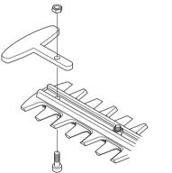
Use the screw and the nut on the cutting deck. Tighten to 8 Nm.
