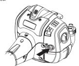
**Choke:** Set the choke control in the choke position.
