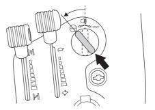
3 When the Rider is at a standstill, press down the parking brake and push in the locking button.
