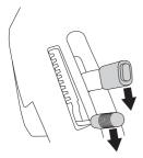
3 Push the equipment frame down and place the catch against the frame.
