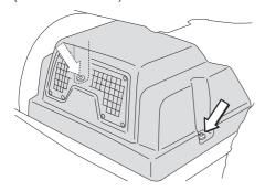
2 Check that there is oil in the transmission's oil tank.
