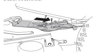
3 Undo the nuts on the lift strut.
