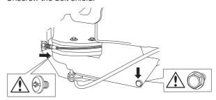
2 Lubricate using a grease gun, 1 nipple from the right-hand side under the engine's lower belt pulley, until grease is forced out.
