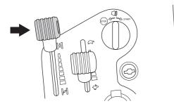
8 Let the engine run at moderate speed or half throttle for 3-5 minutes before subjecting it to heavy load.
