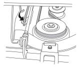
3 Tension the belt with the belt adjuster.
