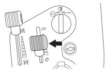
9 Set the required engine speed with the throttle control.
