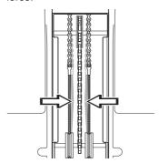
3 If necessary, the wires can be adjusted by tightening the adjuster nuts on each side of the steering collar.
