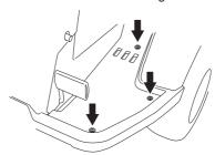
2 Loosen the locking nuts (1).
