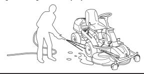
IMPORTANT! Always park the machine on a level surface with the engine OFF before performing any maintenance.
