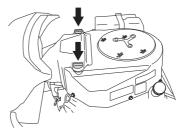
2 Loosen the hose clip that holds the filter cartridge.
