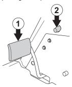
2 Carefully press down one of the pedals until the required speed is obtained. Pedal (1) is used to drive forwards, and pedal (2) to drive backwards.
