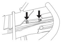
4 Screw out (extend) the stay to raise the rear edge of the cover.
