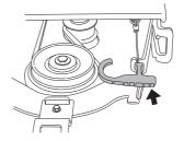
5 Loosen on the cutting height stay and place in the holder.
