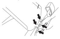
7 Refit the cables and screw the lamp holder on to the servo housing.
