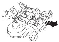
8 Lift the unit until it stops and a clicking sound is heard. The unit locks automatically in the vertical position.
