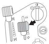
4 If the engine is cold move the choke lever backwards to its end position.
