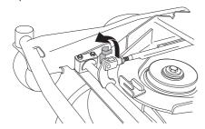
3 Unscrew the bolts holding the unit frame bracket.
