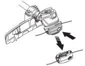
Pull out the line chute assembly.
