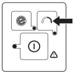
When the rotation button is pressed, the green diode will lit and the trimmer head rotates in counterclockwise. The trimmer head always rotates clockwise by default (green LED is off).
