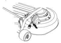
5 Put the lifting lever in the mowing position.
