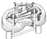
6 Tension the belt with the belt adjuster.
