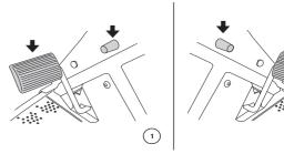
3 Rider 112C has the brake pedal and lock button on the left hand side. (1) Rider 112C5 has the brake pedal and lock button on the right hand side. (2)
