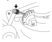
In order to obtain an even cutting height, it is important that the air pressure is the same in both front wheels. See the "Technical data" section.
