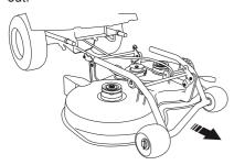
10 Lift off the deck and lean it against the machine or a wall.
