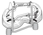
Lock the blade with a wooden block. Loosen the blade bolt and remove the blade bolt, the washer and the blade.
