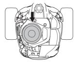
A blocked cooling intake will interfere with the cooling of the engine, which can damage the engine.
