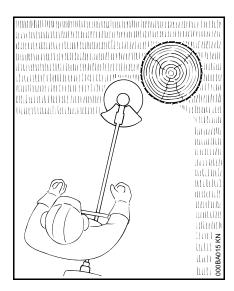
Nylon line achieves a soft cut for edging and trimming around trees, fence posts, etc. – less risk of damaging tree bark.
