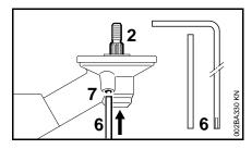
The output shaft (2) must be blocked with the stop pin (6) or screwdriver (6) to mount or remove cutting attachments. These parts come standard with the machine or are available as special accessories.
