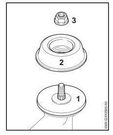
Depending on the cutting attachment, it may be necessary to use the nut (3) and rider plate (2). The thrust plate (1) must be used with all cutting attachments.
