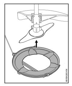
Fit the transport guard on the cutting attachment from below.
