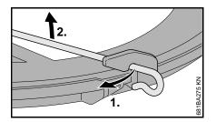
Disconnect wire rod from the transport guard.
