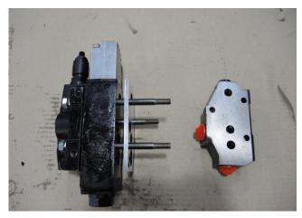
3. Fit the spacer to the main valve checking all Orings are in place. (Item 2)
