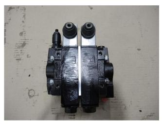
6. Remove the 2 allen bolts in the leaver housing and reverse the leaver so that the leaver point out from the back of the valve.
