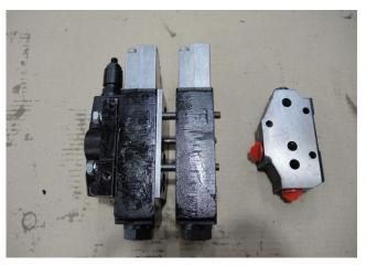
4. Fit the additional valve to the main valve checking all O-rings are in place (Item 1)
