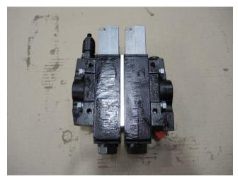
5. Fit the M8 nuts and spring washers and tighten up.
