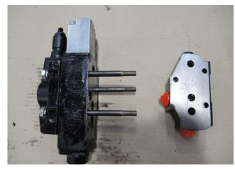
2. Carefully remove the end cap from the valve, making sure the O-ring stay in place
