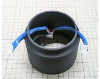
3. Attach the boss cover to the boss body and at the same time attach the genuine harness 12-pole coupler.
