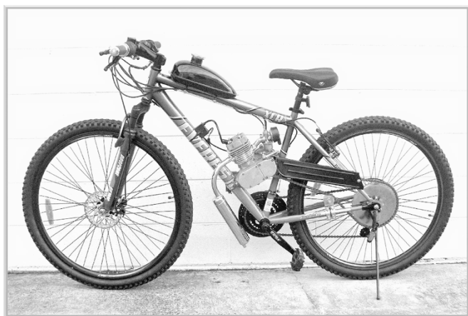
The over-sized ‘Down Tube’ & large number of Spokes makes this “Everest” installation a challenge
