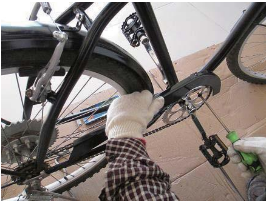
Step 16. Engine installation, find 8 of the 6*55 double headed screws and insert to the front and rear-mount, then tighten the screws.
