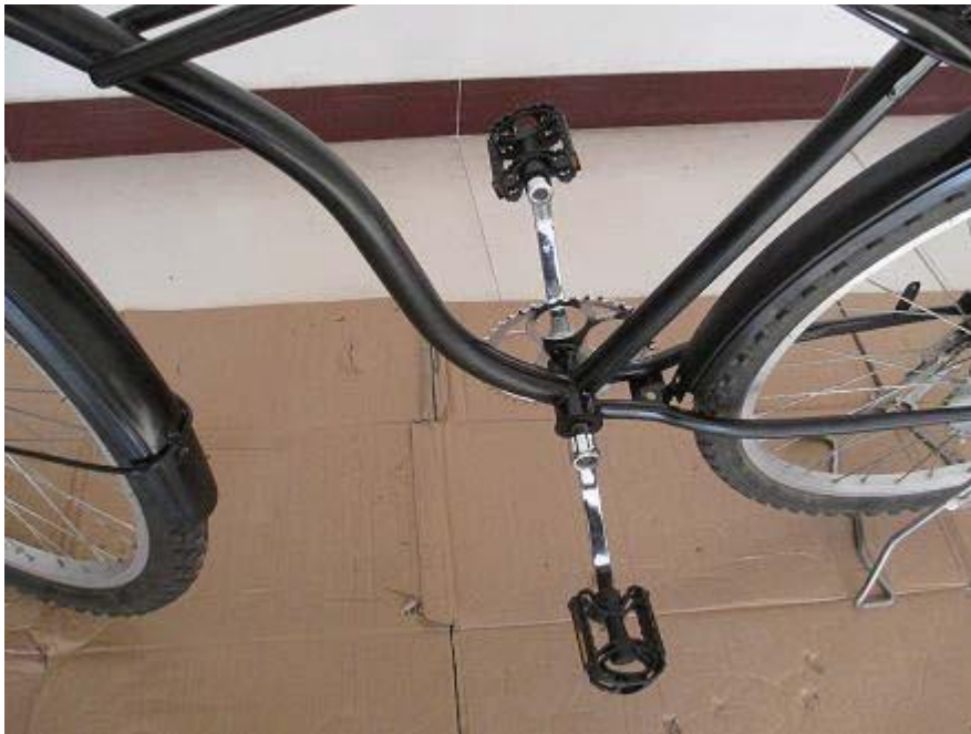
Step 15. Install the original chain to the new chain crank.
