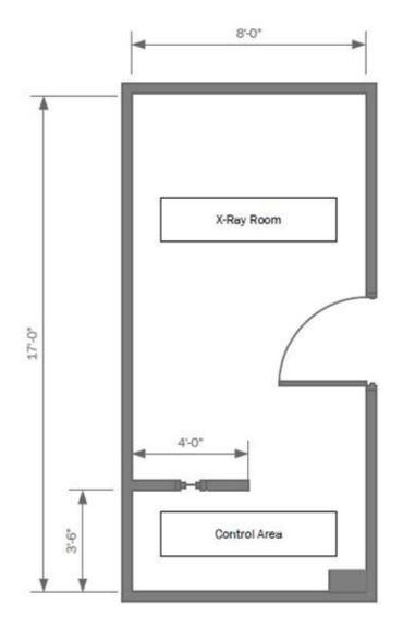
Maven Imaging provides room drawing as part of the purchase of any X-ray room installation. Complete room layout with all the electrical requirements and information to pass to a physicist for the shielding report.
