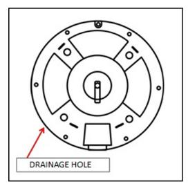
rainwater from entering through the hole. To drain the boat, simply turn it on its side, so the hole is directly over the ground, and tilt the boat until water begins to drain out. Contact us if you need further instructions.
