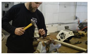
The old bearing races are removed by simply using a punch. The copper jaws on the vice help to avoid damaging any parts that are held.
