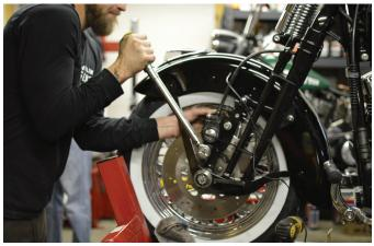
With the fender and wheel back in place Kekoa puts the final torque on the caliper bolts before pulling this bike off the lift.
