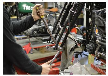
The reassembly is very simple but always take the time to properly torque the fasteners to factory specs.
