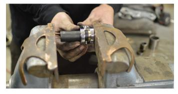
There are two more bearing races that must be pressed into the rockers. Kekoa uses a deep well socket to reach inside the rocker and press the race in the vice.
