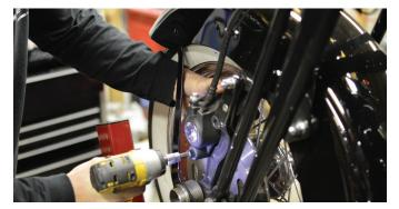
The rotor is easily removed by simply extracting the two mounting bolts
