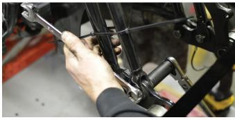
Kekoa uses Zip ties to secure the legs prior to removing the rockers. This is done to ensure that the front leg of the springer does not decide to become a projectile weapon.
