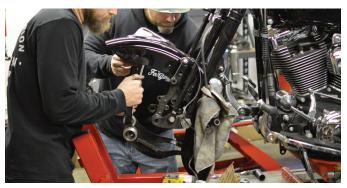
Although one person can certainly complete the job it is always nice to have a second set of hands when handling painted surfaces. The front fender is carefully maneuvered out from between the front legs of the springer.
