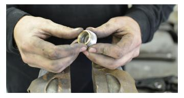
The kit provides brand new shiny bearing races which must be pressed into each side of the threaded bearing retainers. Be sure that the races are facing in the proper direction before pressing them into place.
