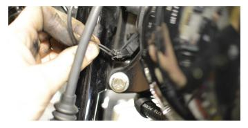
Before removing the front fender, Kekoa unplugs the wiring to the indicator light located on top of the fender.
