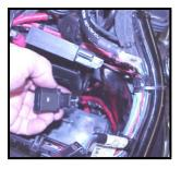
**FX/FLST-J:** Position rear oxygen sensor harness connector on top of oil tank, just forward of the battery under battery ground cable as shown.
