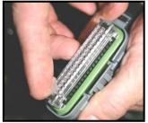
Also apply dielectric grease to the ThunderMax oxygen sensor harness connector terminals to help maintain vital conductivity, and to the outer housing to prevent binding upon installation to the ECM.
