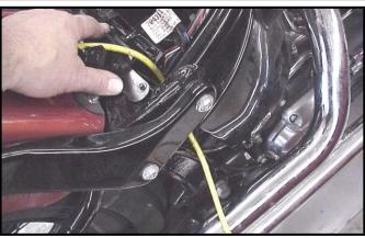
**FX/FLST-G:** Install the ThunderMax ECM onto the ECM caddy studs without nuts; insert the oxygen harness connector into the ECM with the imprinted "ThunderMax" logo facing up. Tighten the (2) Phillips connector screws. Lift ECM and install main 36-pin connector, ensuring it is fully seated and latched. Replace ECM onto studs.
