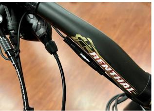
**1.11** Configure the cockpit and clean up the wiring like in the photo below. Use the supplied Velcro straps to keep the wires neat and out of the way when you turn the handlebars
