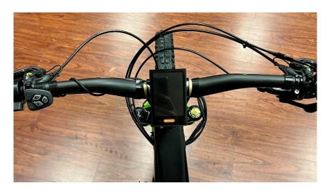
**1.13** Make sure the display is plugged into the main wiring harness. The green triangular connector on the 750W/1200W will be by the handlebar and plugs directly into the back of the display. The display connector for the 1600W can be found on the right side of the headtube as shown.
