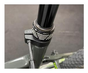
**1.9** Install the saddle onto the dropper post. Place saddle rails into clamp, adjust angle and fore/aft position per bike fit, and tighten bolts with 5mm allen wrench to 8-10NM
