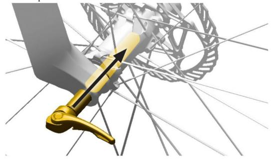
**1.4** To tighten the Maxle into the drop out, turn the lever clockwise until there is a small gap between the lever head and drop out
