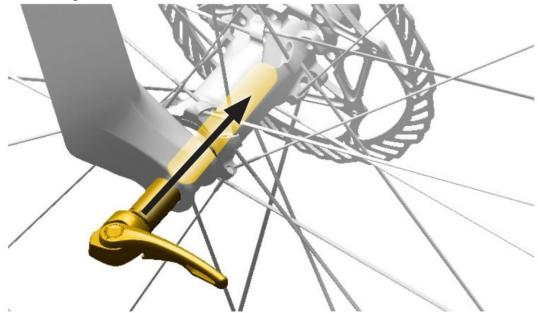
**1.4** To tighten the Maxle into the drop out, turn the lever clockwise until there is a small gap between the lever head and drop out
