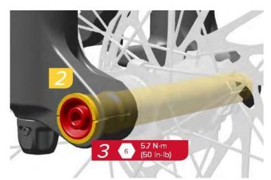
Step 2 and 3: Install the Maxle through the drive side dropout then tighten to 50 in-lb (5.7Nm)
