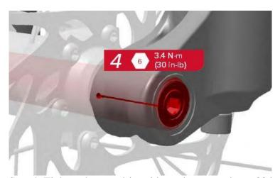
Step 4: Tighten the non-drive side wedge expander to 30 in-lb (3.4Nm).
