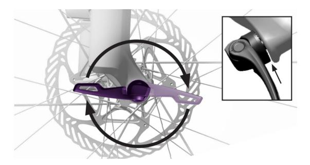
**1.6** Close the Maxle lever. Lever tension is sufficient if the lever leaves an imprint on your hand. To increase lever tension, open the lever and turn it clockwise. Close the lever to recheck lever tension. Repeat until the tension is sufficient, then close the lever. When the lever is closed, verify there is no gap between the lever head and dropout.
