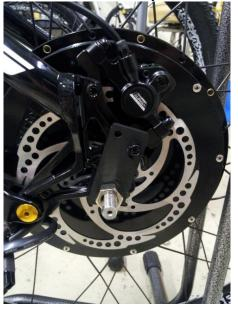
12. Install throttle as pictured. You will need an Allen wrench to adjust the throttle and also the brake assembly of your existing bike. You can cut your existing hand grip as needed to match your left hand grip.
