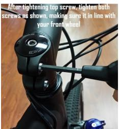
Now you can unscrew the 4 screws on the front of the stem which will hold the front handlebars in place. Secure the handlebars using the 4 screws and make sure it is lined up in the middle. After this, it is **VERY IMPORTANT** to go back and screw the 3 screws on the other end of the stem and make sure the handlebars are aiming straight in line with the front tire. Tighten the top screw first, followed by tightening the 2 on the side.
