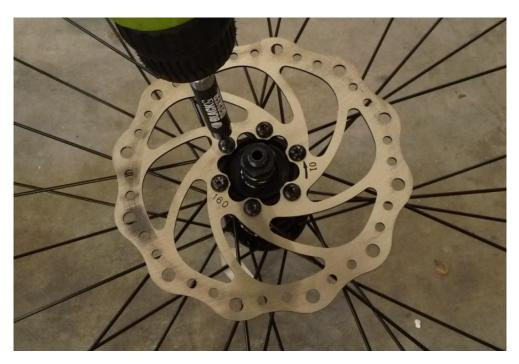
4. Screw disc brakes (if applicable) onto the motor wheel. Use included disc spacer washers if necessary. You can move the disc outwards by placing the washers on the inside (underneath) the disc. For geared motors systems, use 2 washers per screw to allow the bolts to seat flush inside the disc motor mounts.
