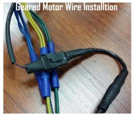
2a) Geared motor systems will have **3 phase wires and a 5 pin hall sensor connector** coming from the motor. After matching the phase wires color to color, make sure you plug in the 5 pin hall sensor connector. Some of our higher power 5000W and 6000W gearless systems (Crystalyte type motors) have a **round 5 pin hall sensor** as well. Make sure to plug the mating connector from motor to controller.
