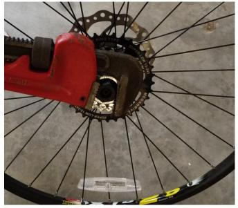
6. Spin Freewheel onto the hub motor. For our GEARLESS motors, you may be required to add a spacer washer between the hub and freewheel if you did not purchase the freewheel installed from HPC
