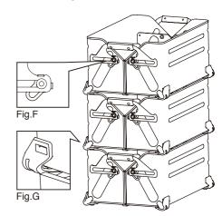
Check that all of the locking pieces are as shown in Fig. F. Check that all of the main feet of the stacked units are as shown in Fig. G.
