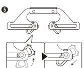
Set the locking units and adjust them as shown above Confirm that all four locking units on both handles are I ocked.
