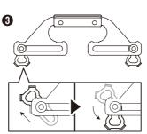
Unlock the four locking units and adjust the handles as shown above. If the locking units are not firmly facing downwards, the pieces will interfere with one another when the box is opened or closed.
