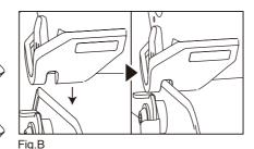
tack the units on top of each other ensuring that the main feet on the box being stacked on top are properly engaged with the unit below it, (as shown in Fig. B).
