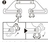
Unlock the four locking units and adjust the handles as shown above. If the locking units are not firmly facing downwards, the pieces will interfere with one another when the box is opened or closed.
