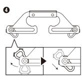
Set the locking units and adjust them as shown above. Confirm that all four locking units on both handles are locked.
