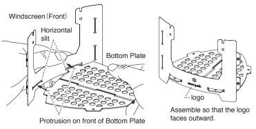
⚠ CAUTION If it is difficult for the protrusion to enter the slit, turn the Windscreen at an angle and insert the protrusion.
