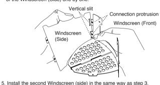
1) Make sure that the side with the concave protrusions is facing outward. 2 Make sure that the horizontal slit of the Windscreen (Side) is facing down. 3 Insert the protrusion on the side of the bottom plate into the horizontal slit of the Windscreen (side).
