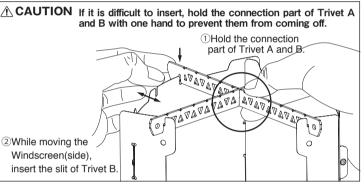
11. When Trivet A and B are firmly inserted into the Windscreen (Front, Side), it is completed
