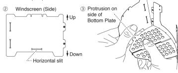
4.Insert the connection protrusions of the Windscreen (Front) into the vertical slits of the Windscreen (Side) one by one.
