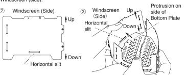
6.Insert the connection protrusion of Windscreen (side) into the vertical slit of the Windscreen (side)
