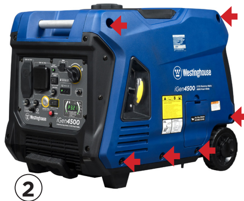
2 Remove 6 10mm bolts that hold on side panel
