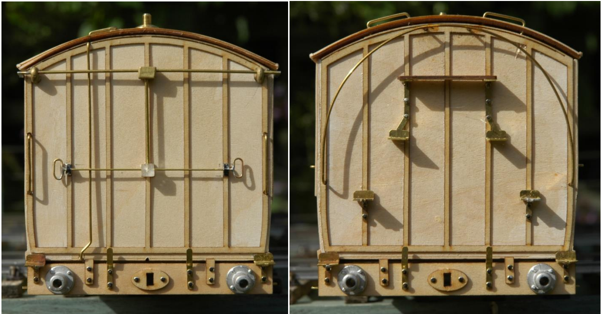
Communications, steps and handrail
