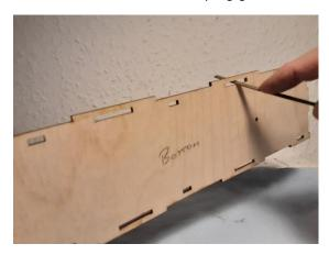
Apply PVA to the top edge of the Solebar, press into position fully against the underside of the floor and weight or clamp to a flat surface and allow to dry.
