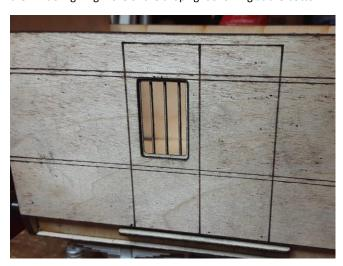
The end details can now be added. First the Drop plates are added. These are positioned centrally with the bottom edge lined up to the top end of the Headstock.
