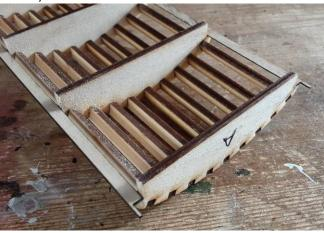
The Roof Covering are now fitted. The central sheet needs to be formed to be an easier fit onto the roof structure. This is done by soaking the sheet in warm water for at least 30 minutes and then strapping to a piece of tube. When the sheet dries out it will have taken a curved form and be easier to fit on the roof structure.
