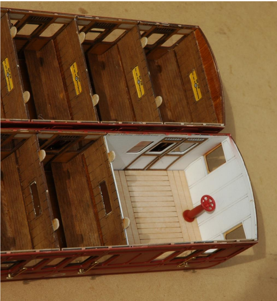
There are slatted seats and a boarded floor overlay for the guard/baggage compartment.
