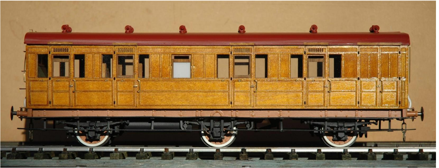
ECJS D.1/GNR D.164C Semi-corridor lavatory composite with baggage compartment
