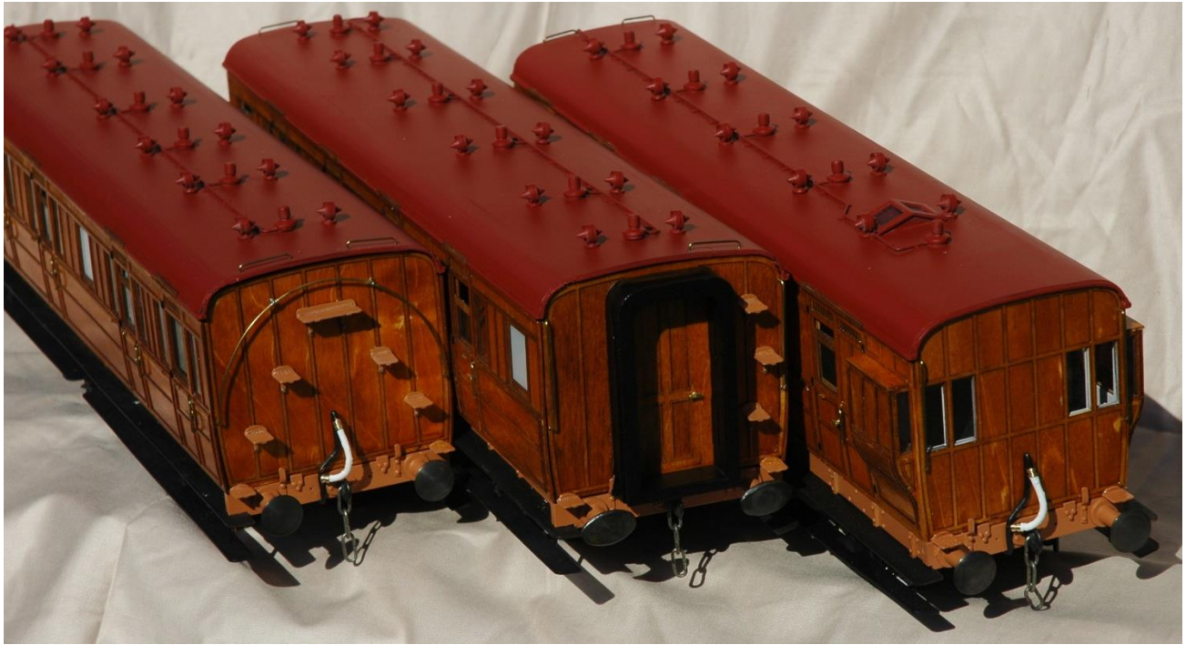
Carriage ends showing steps, corridor connector, vacuum hoses and handrail
