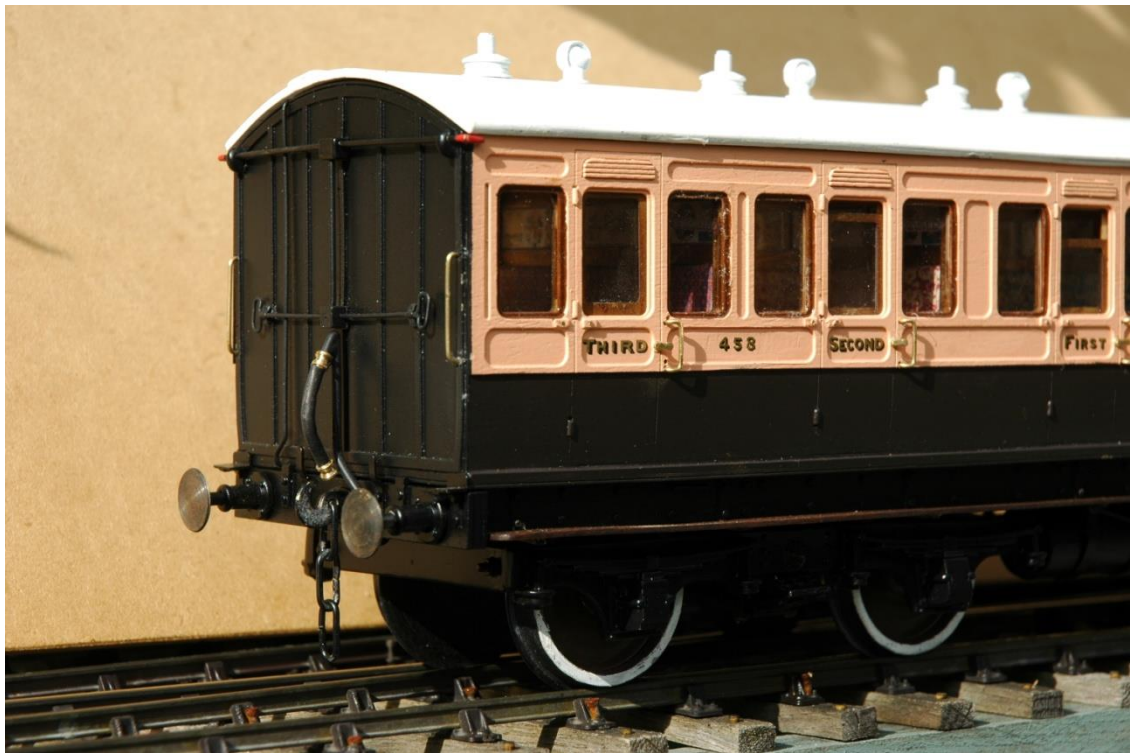
Communication end of the 45ft brake composite carriage
