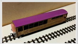
This is a multimedia kit designed to run on 9mm gauge track. It is based on the modern Ffestiniog Railway Coaches as operating today as part of normal service trains. This kit is for the Coach Number 114 from the 'Carnforth' Design Series.
