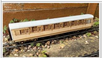
This is a wooden kit designed to run on 12mm gauge track. It is based on SR Maunsell Restriction 1 Corridor Composite Coach.
