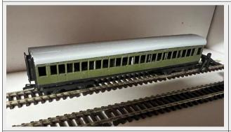
This is a wooden kit designed to run on 12mm gauge track. It is based on the SR Maunsell Restriction 1 Corridor 3rd Coach.
