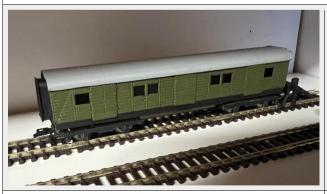
This is a wooden kit designed to run on 12mm gauge track. It is based on the SR Corridor Bogie Luggage Van.
