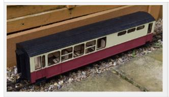
This is a wooden kit designed to run on both 32mm and 45mm gauge track. It is based on the modern Ffestiniog Railway Coaches as operating today as part of normal service trains. This kit is for the Buffet Coach Number 114 from the 'Carnforth' Series.
