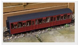
This is a wooden kit designed to run on both 32mm and 45mm gauge track. It is based on the modern Ffestiniog Railway Coaches as operating today as part of normal service trains. This kit is for the Composite Coach Number 104 from the 'Barn' Design Series.
