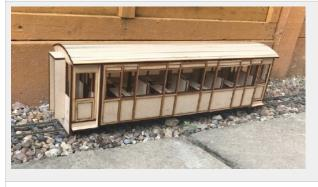
This is a wooden kit designed to run on both 32mm and 45mm gauge track. It is based on the modern Welsh Highland Railway Coaches as operating today as part of normal service trains. This kit is for the Shortened Saloon Coach.
