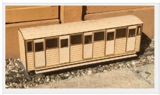
This is a wooden kit designed to run on both 32mm and 45mm gauge track. It is based on the preserved Chattenden and Upnor Railway Coaches as operating today on the Sittingbourne and Kemsley Light Railway. This kit is for the Former Coach Number 204.
