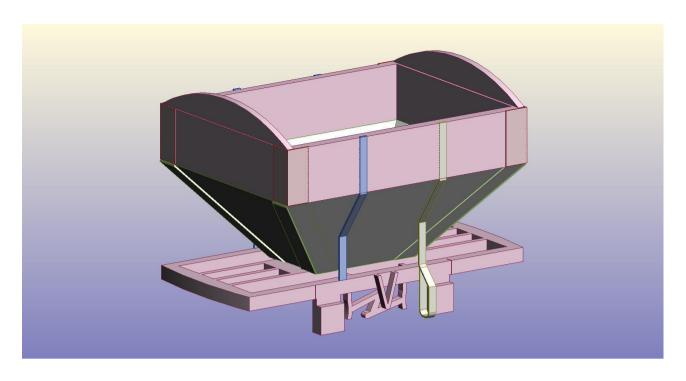
Next, glue into place the side strapping. The brake unit going on the side with the V hanger.
