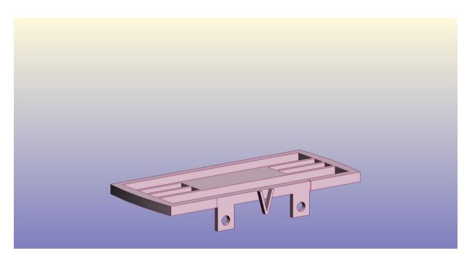
To start on the brake rigging, glue the V hanger on the outside of the model.
