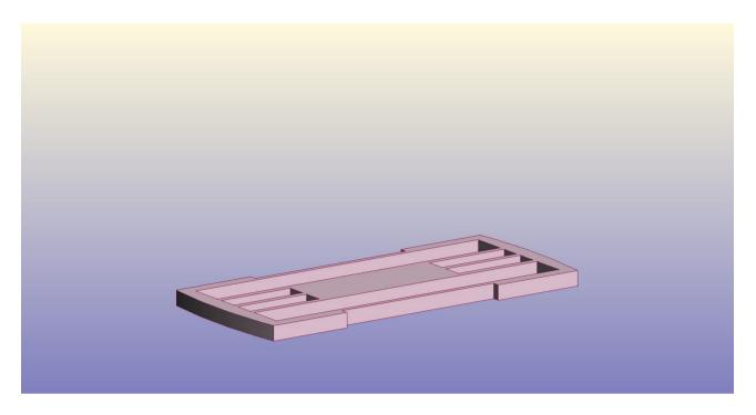
Start by gluing the two chassis plates together on top of each other.
