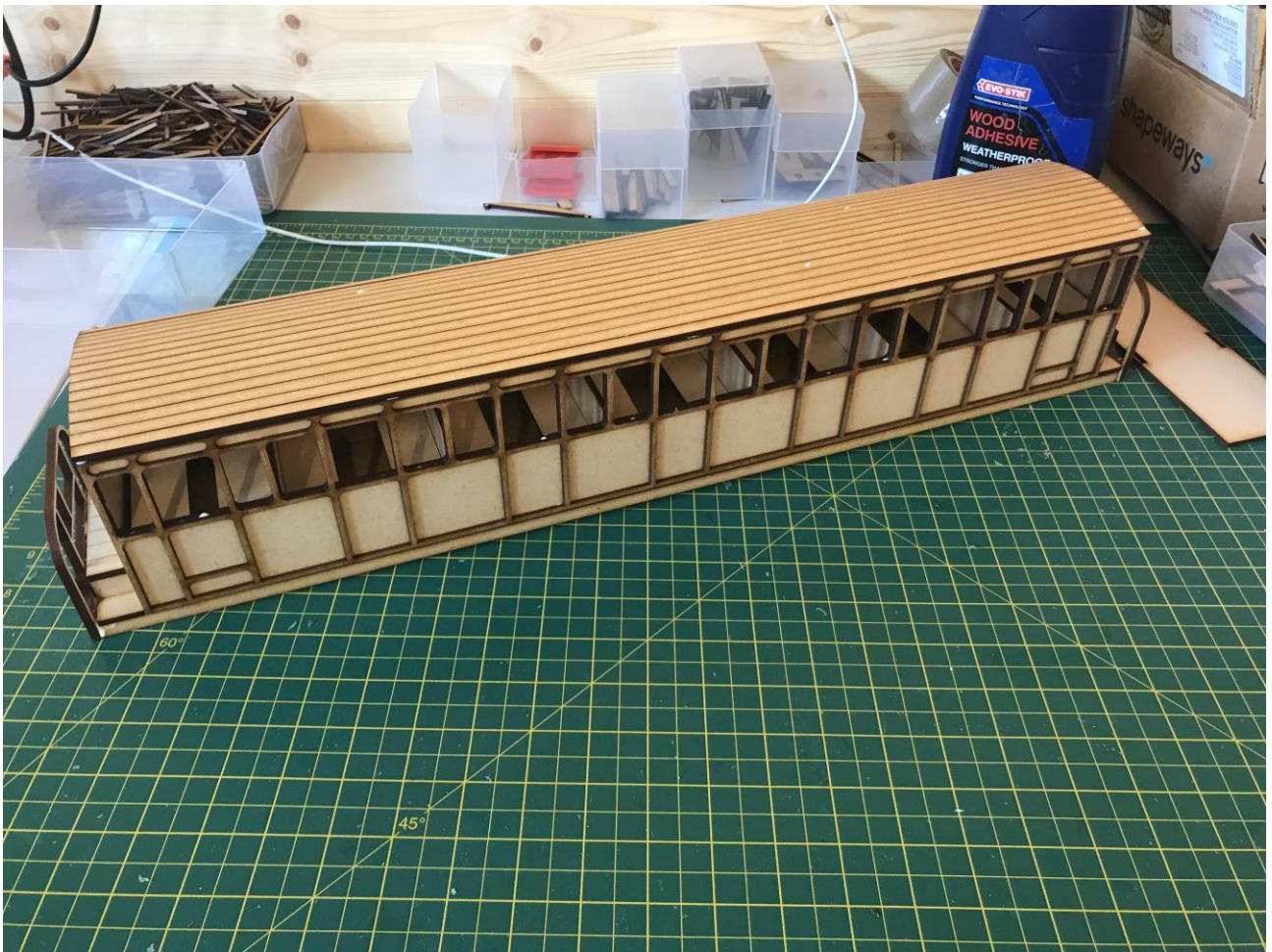
Now its time to glue the roof on. The roof beams sit on the top of the coach.
