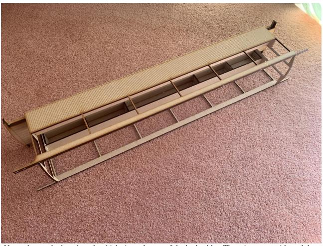
Next, glue on the long boards which sit on the top of the body sides. There is one per side and they sit within the etched line on the body side.
