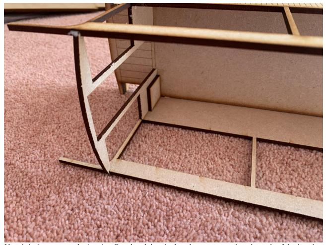
Now it is time to start the interior. Start by gluing the bench supports against the ends of the interior. Repeat for all 4 corrners.
