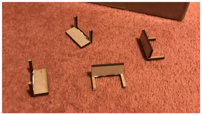
With the bogies installed, time to add the steps. Glue the U shape parts of the step to the step plank to make a L shape.
