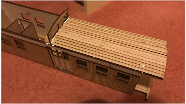
Glue the first side of the Cuplola on the roof. These sit on the sides of the model and flush with the roof section already installed. We recommend adding this part and the parts mentioned in the step before at the same time.
