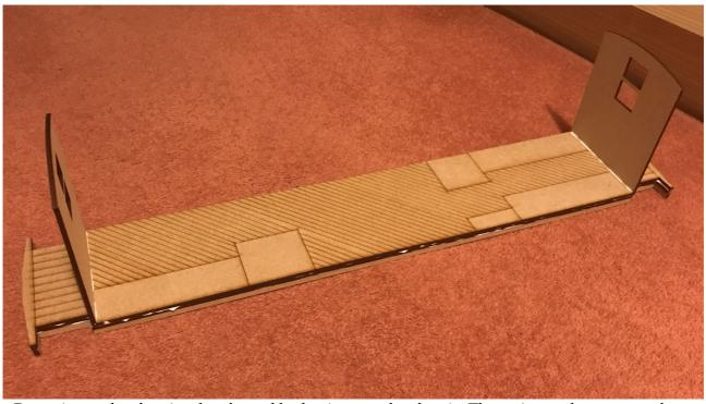
Returning to the chassis, glue the end body pieces to the chassis. These sit over laser cut marks at each end of the main chassis.
