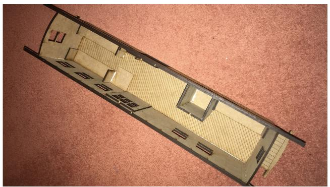
Interior time. Glue the uprights inside the body. These sit inside the long thing sections laser etched on the floor. It is now the best time to glue the toiler compartment in place.
