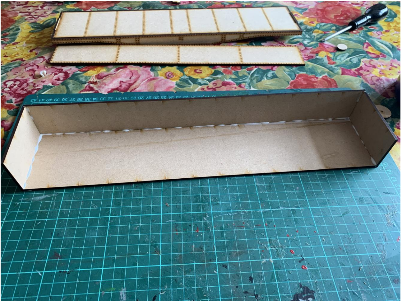
Tank Wagon – Start assembling the tank by gluing one of the sides and the two ends onto the tank top.
