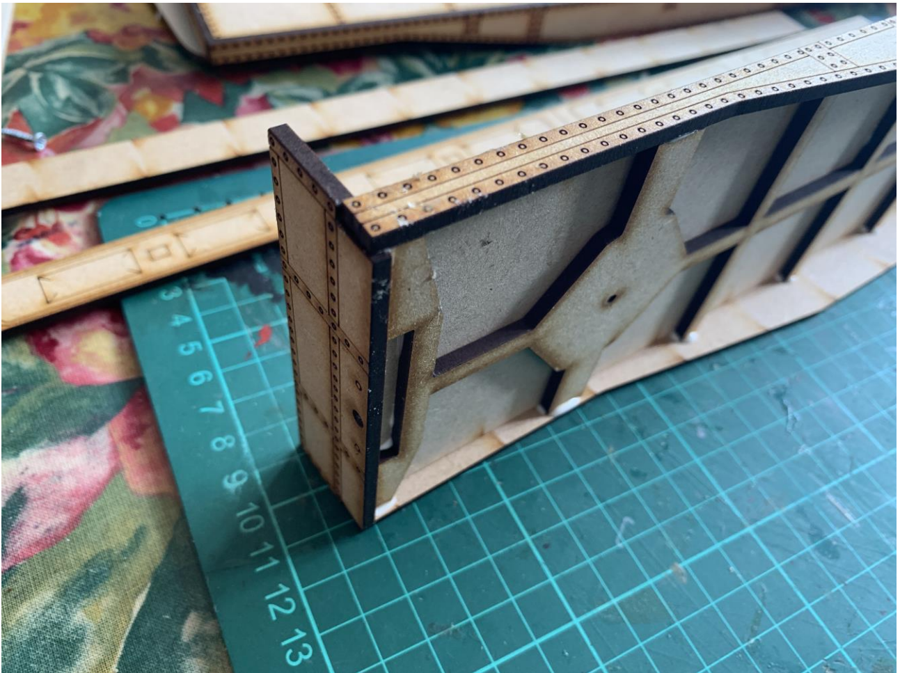
Coke Wagon – This kit features a different buffer beam which slots over the top of the chassis side panels. This also has the coke wagon end panel included forming a combined headstock.
