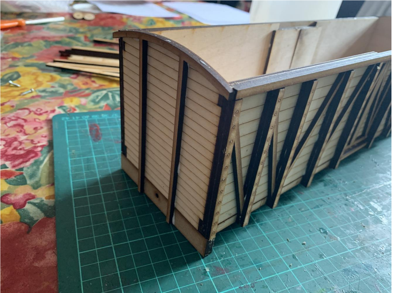
The final step before going on the roof is gluing on the van end beading which sits on the ends of the van level with the top of the curved section.
