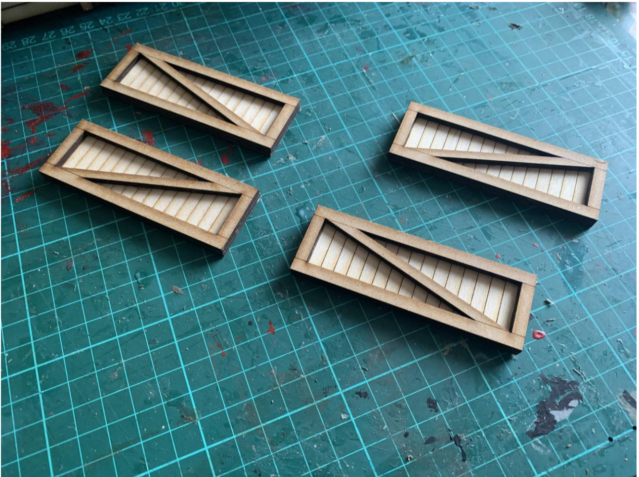
The doors are formed of a framing section and the door panel itself sitting underneath. There are 4 doors in total which are paired.
