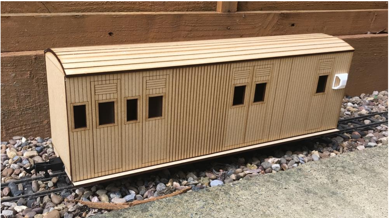
On the V5 and V16, the brake ducket is glued approximately 3/5ths of the way up the model at the end of the coach. This is the end furthest from the double doors on the V16 and closest to the single door on the V5.
