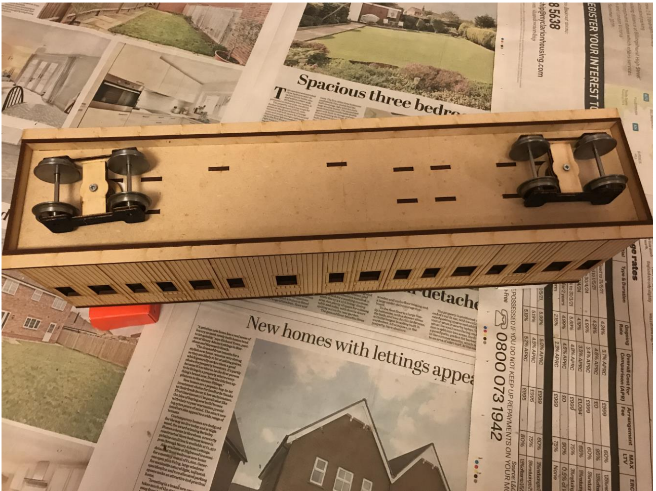
Time for the bogies to be installed. These sit approximately 2 inches from the end of each coach. These give a prototypical location and allow for maximum movement of the bogies on curves.
