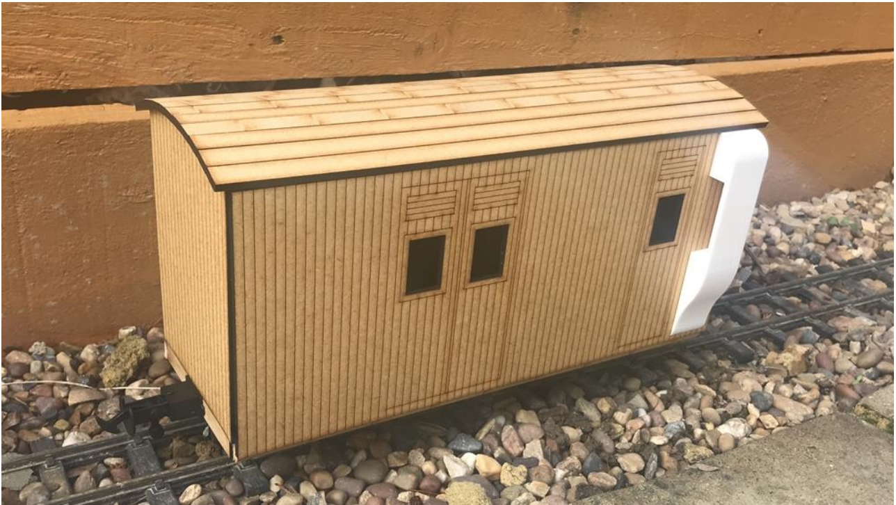
On the V2 and L4 brake vans, the duckets are glued on the ends of the coach between the single door and the end of the vehicle.
