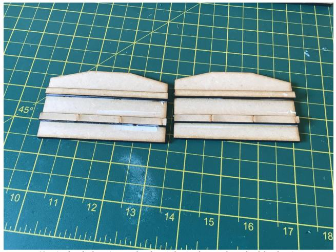
Now is also the best time to glue the reinforcing bars to the ends of the chassis.
