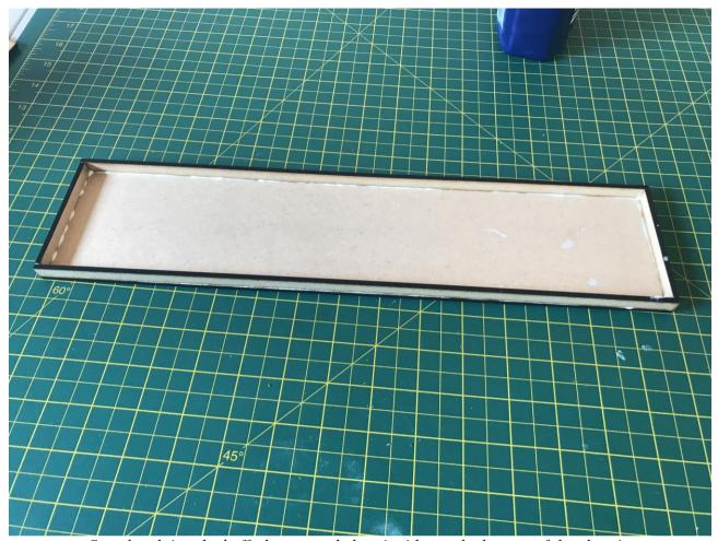
Start by gluing the bufferbeams and chassis sides to the bottom of the chassis.
