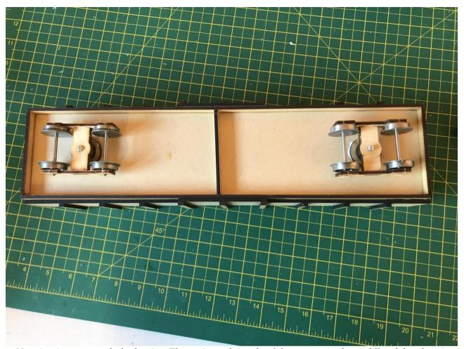
Now its time to attach the bogies. These sit on the ends of the wagon in the middle of the chassis approximately ½ a wheel diameter inside the chassis. Once these have dried, glue the couplings on the ends of the wagon in the middle of the body. This completes the wagon.
