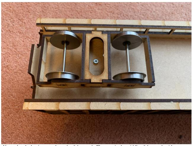
Next, glue the bogies onto the ends of the coach. These go in the middle of the coach with room to swing around curves.
