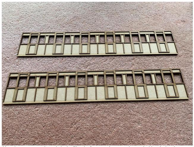
Now time to start on the main body. Glue the 2mm overlays onto the coach sides placing them over the top of the etched lines on the sides.
