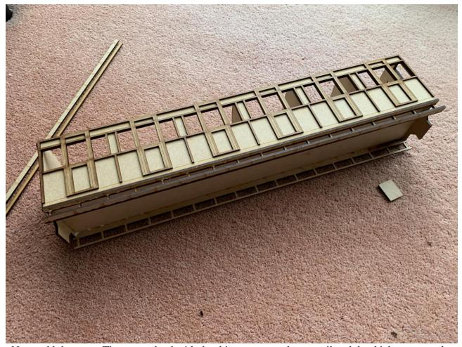
Next, add the steps. These are glued with the thinner one on the top rail and the thicker one on the bottom rail. To help identify these from the roof beams, these are shorter in length and there is 4 of them in total (2 thin, 2 thicker)
