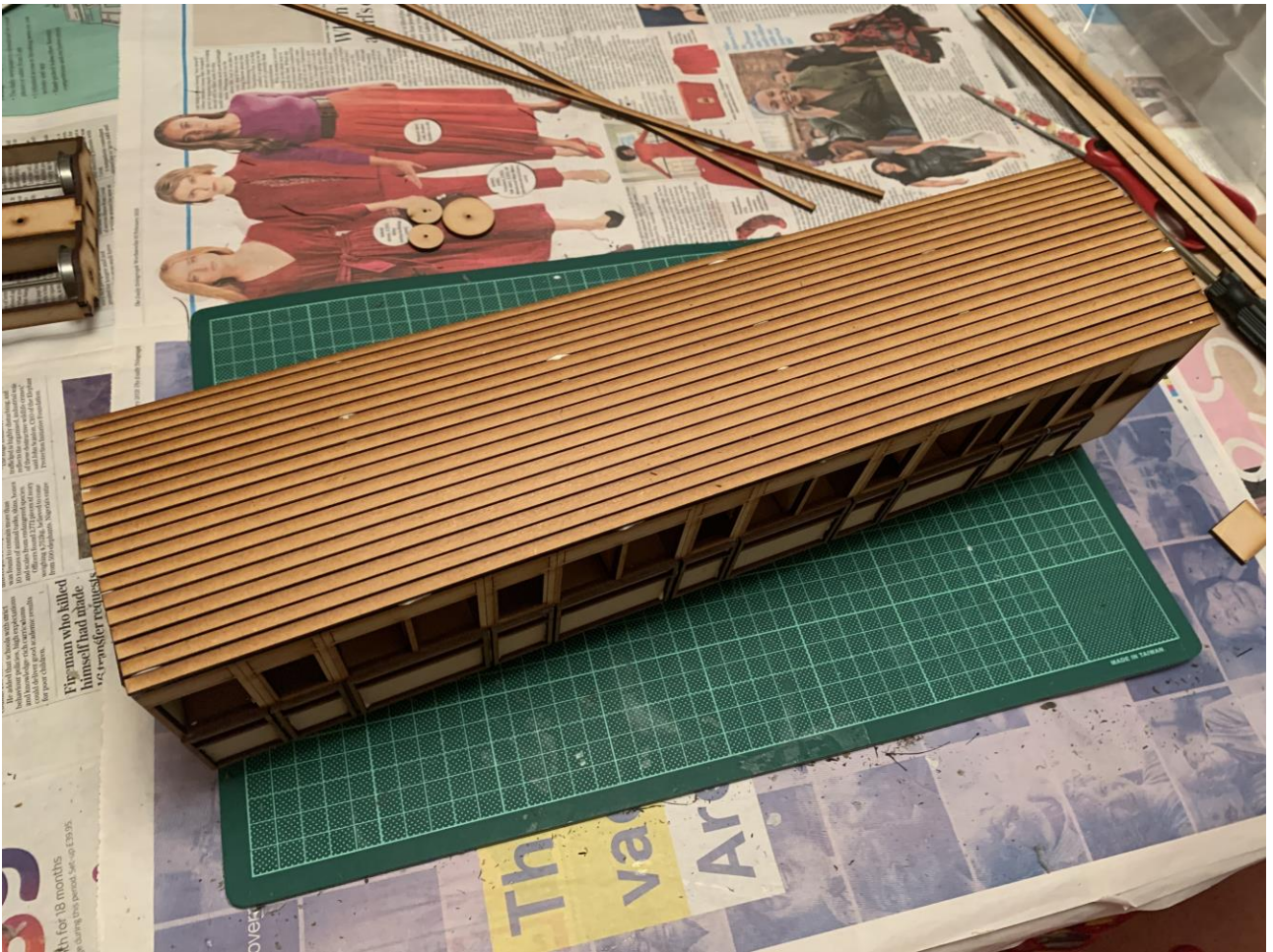
Now glue on the roofbeams. These run the length of the coach including over the beading on the ends of the coach.
