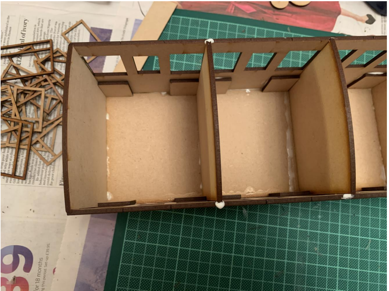
Start assembly of the seats. One seat support goes in the corner of each compartment on the coach.
