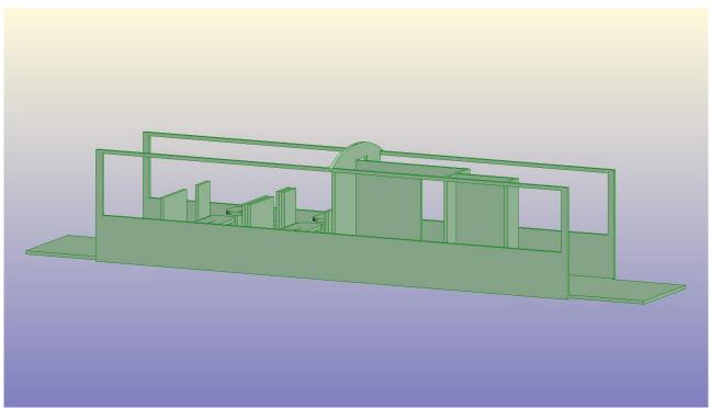
To start assembling the main body, glue the inner layer of the body side onto the lip between the side of the tables/seats and the edge of the chassis plate. For reference, these are the shorter of the four main body sides.
