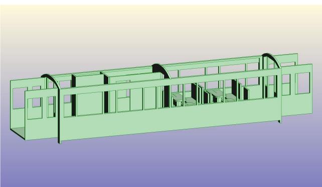
*Next, glue into place the doors. The smaller of which are closest to the passenger compartment.*
