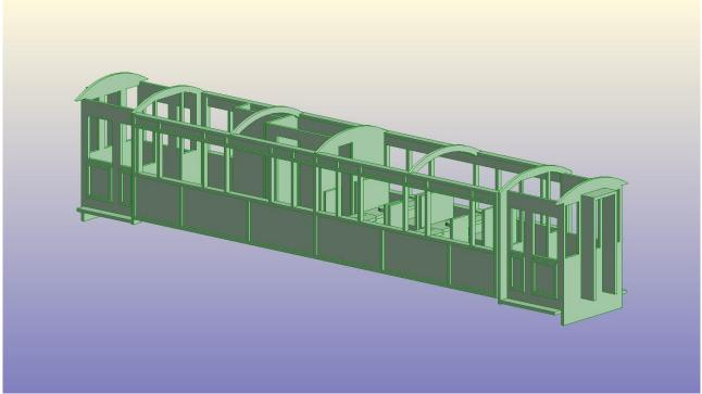
Before installing the roof, a small number of roof supports need to be glued into place. Where you place these is your choice but we recommend placing them equally along the roof
