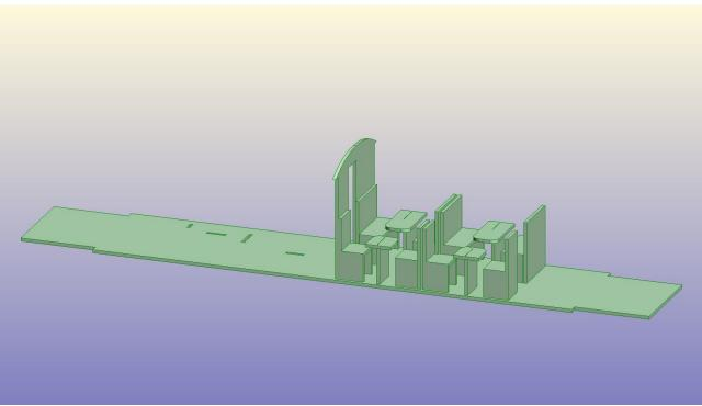
To complete the interior, glue in the internal partition into place at the end of the seating area.
