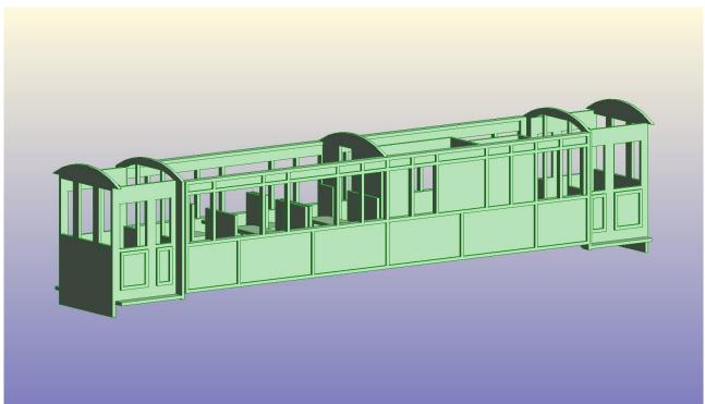
Now its time to glue on the beading. To aid you, there is etched markings on the sides and ends of the coach to show you where they go. Note, each side is different to each other.
