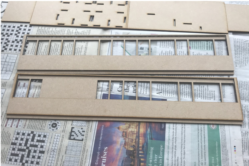
The sides simply attach onto each other. The same gaps are on the sides (3mm each side) with the top being a flush fit. The interior pieces also double up at the mounting points for Window Glazing.
