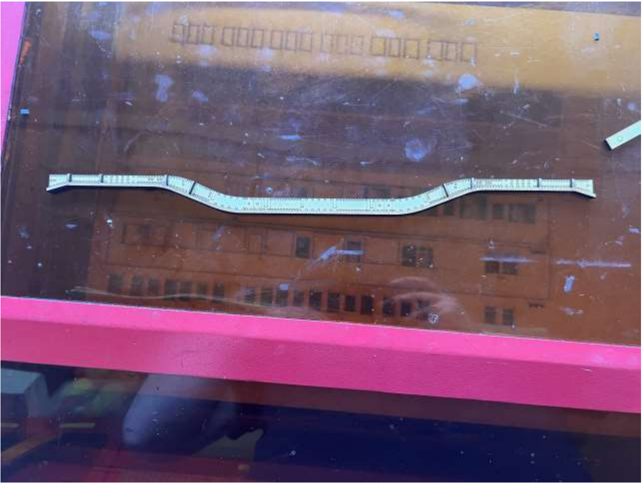
First, glue on the bottom bar of the wagon side.
