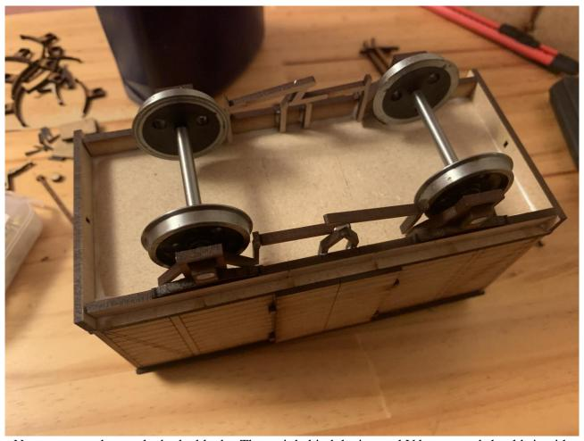
Next you can glue on the brake blocks. These sit behind the internal V hanger and should sit with the wheels able to turn freely.
