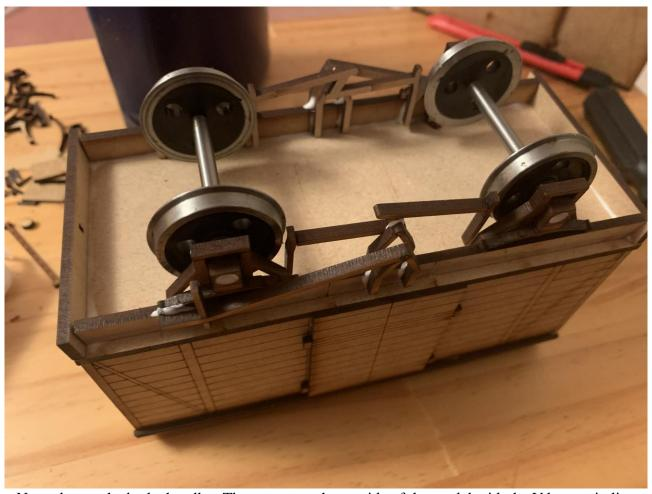
Next glue on the brake handles. These go onto the outside of the model with the V hanger in line with the one on the interior.
