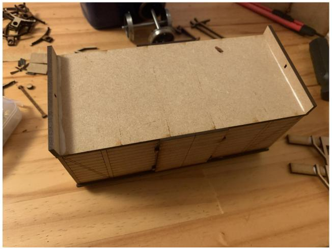
Now, glue the bufferbeams onto the ends of the chassis plate.
