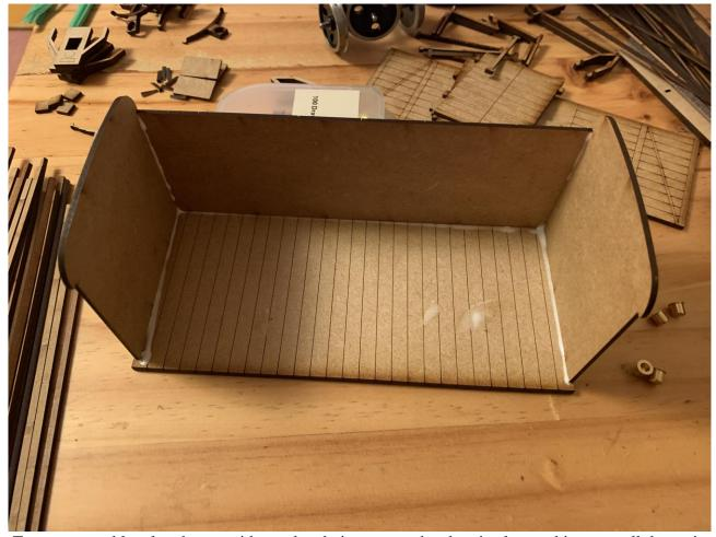
To start assembly, glue the two sides and end pieces onto the chassis plate making sure all the main parts are flush with the sides.
