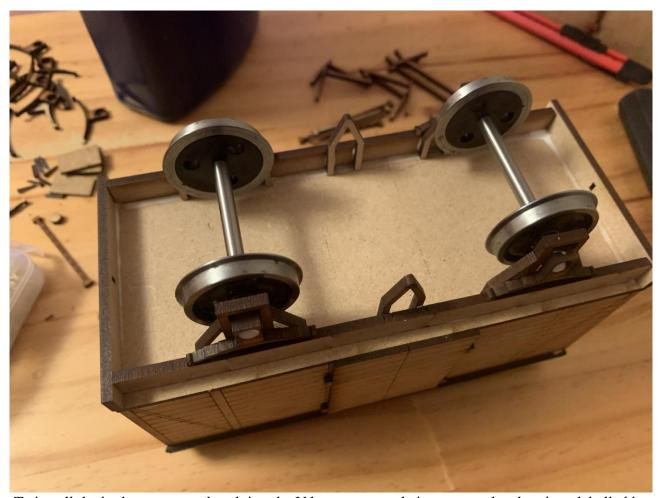
To install the brake gear, start by gluing the V hangers onto their areas on the chassis as labelled by the etched markings on the sides. If you wish to have a wire though the brake gear, you can drill out the etched circle in the centre of each piece for a wire to slide though.
