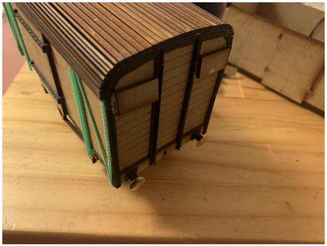
The buffers are formed of two pieces. The first part is to glue on the 3D printed buffer housings into the respective locations as marked on the bufferbeam. For those who wish to use sprung buffers, there is a half etched circle for you to drill though to place the buffers in the correct location. The final stages of the buffers is to glue in the Brass Pins into place to form the buffer unit. Some straightening of the buffers maybe required due to their manufacturing.
