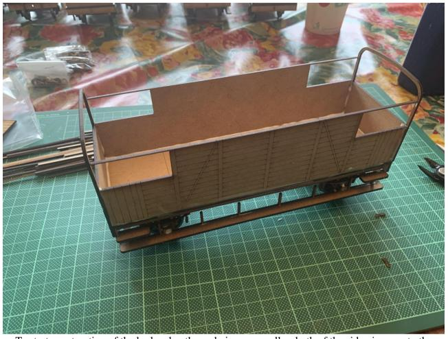
To start construction of the body, glue the end pieces as well as both of the side pieces onto the brake van chassis.
