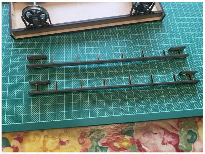
To assemble the footsteps, glue the longer steps on the bottom of the footsteps and the shorter steps to the tops.
