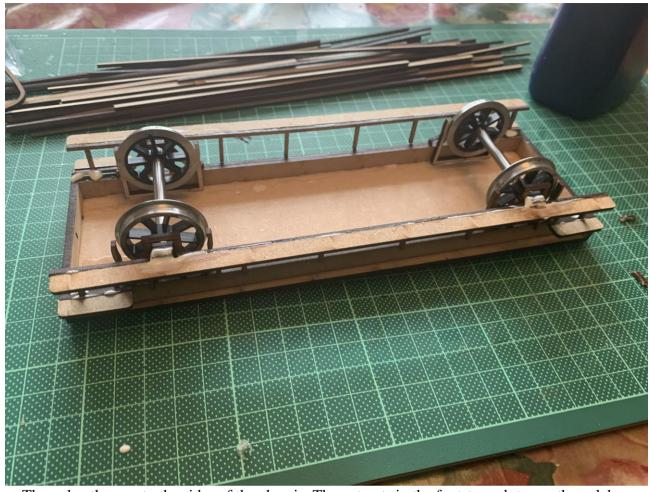
Then glue them onto the sides of the chassis. The cut outs in the footsteps slot over the axlebox covers
