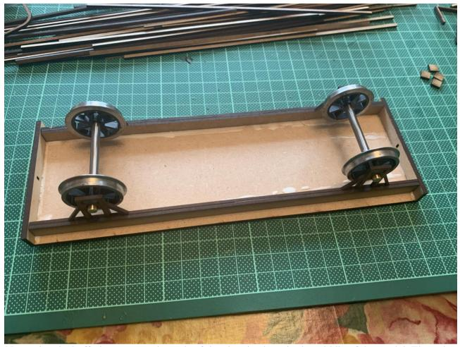
Next, glue the bufferbeams onto the ends of the chassis plates in the middle of the model. Then glue the chassis sides in place while inserting the wheelsets at the same time. This will produce a rolling chassis in a single step.
