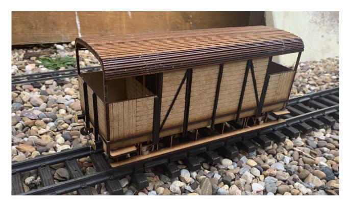
The buffers are formed of two pieces. The first part is to glue on the 3D printed buffer housings into the respective locations as marked on the bufferbeam. For those who wish to use sprung buffers, there is a half etched circle for you to drill though to place the buffers in the correct location. The final stages of the buffers is to glue in the Brass Pins into place to form the buffer unit. Some straightening of the buffers maybe required due to their manufacturing.
