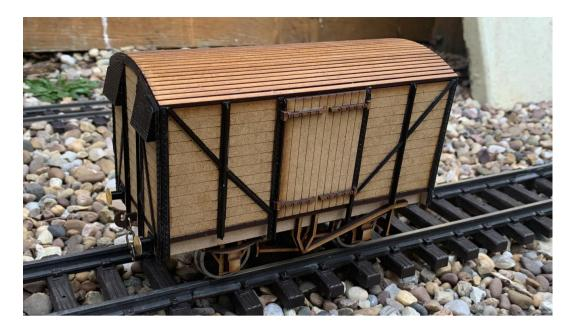
Now its time to start on the strapping. Start by gluing into place the end strapping followed by the side strapping. There is one pair per side on the GWR Van and 2 ends and 2 centre crosses per side on the fruit van. It is also time to glue into place the end strapping on the van as well as the Vents which sit at the tops of the van just inside the strapping.
