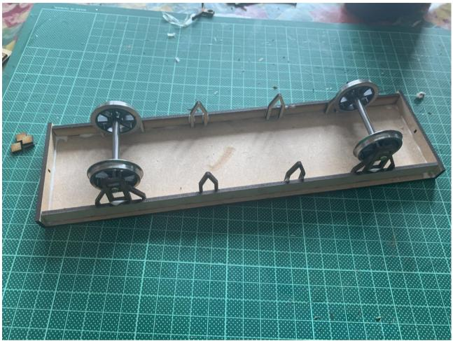
Now, glue the bufferbeams onto the ends of the chassis plate and then glue the chassis sides in place while inserting the wheelsets at the same time. This will produce a rolling chassis in a single step
