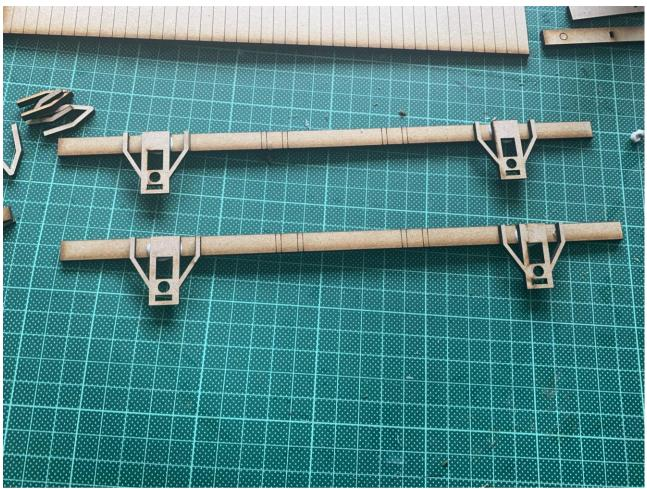
To start assembly of the chassis, start by gluing the axle boxes onto the chassis sides. The sides have etched lines which show the correct location for them on the chassis.
