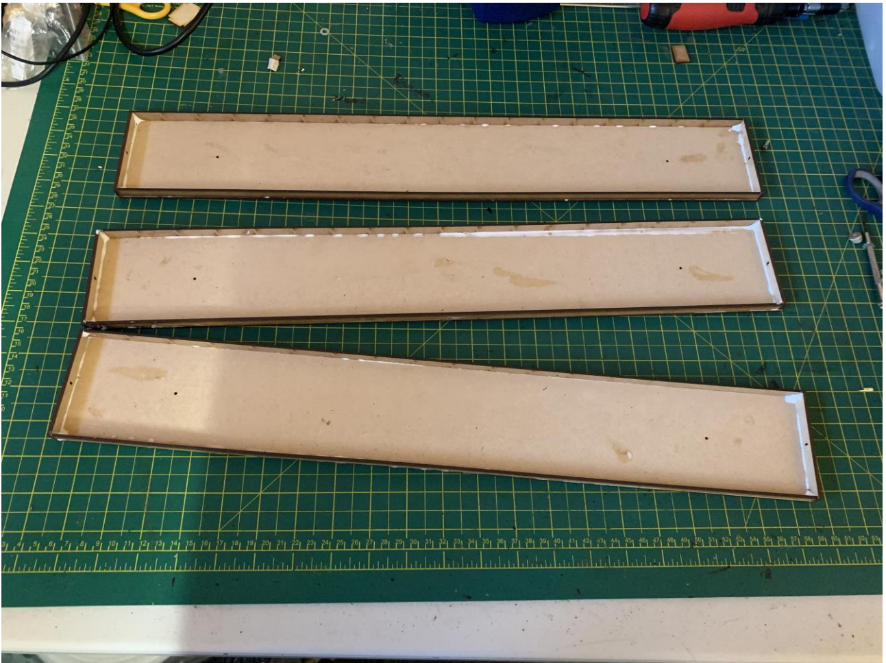
Start by building up the chassis. This is formed of 2 Bufferbeams and two sides per coach.
