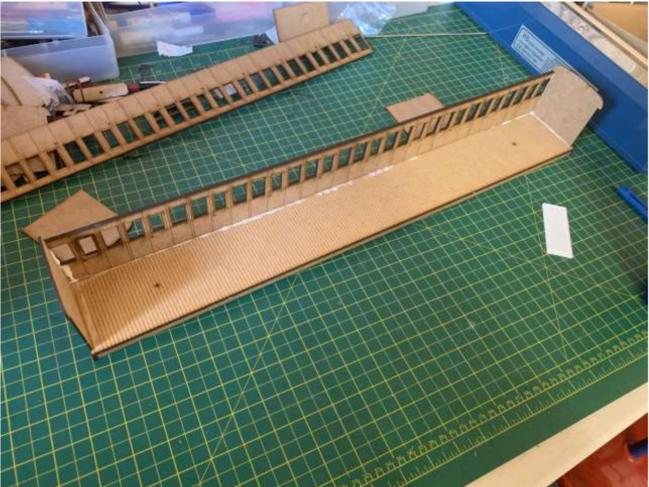
MDF VERSION - Flip the chassis over and then glue one of the coach sides and the two end pieces (the partitions with etched end detail on the outsides) onto the chassis plate.
