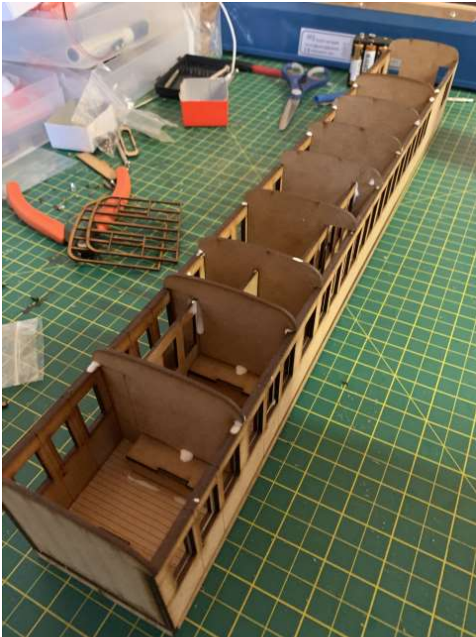
The Composite Brake Coach – Internal Layout. Another view of the internal layout. Note, one of the partitions has a cut out in it for the corridor in that part of the coach.
