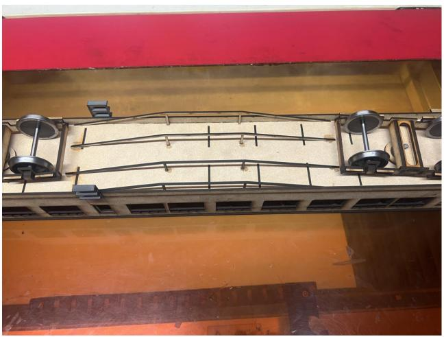
To finish the model, glue into place the Truss Rods. There are 4 in total which are evenly spaced across the body.
