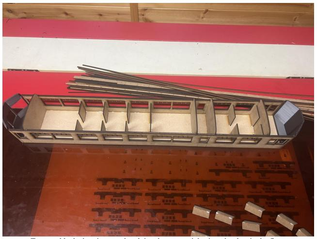
To assemble the interior, start by gluing the seat uprights into the slots in the floor.
