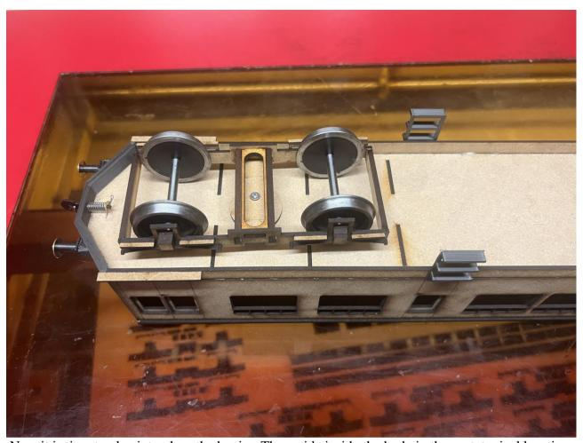
Now it is time to glue into place the bogies. These side inside the body in the prototypical location.
