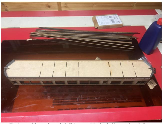
Now is a good time to glue on the bufferbeams and the chassis sides onto the underframe.
