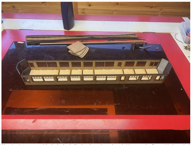
Now its time to assemble the body shell, glue the end panels and sides onto the floor with the etched details facing upwards.
